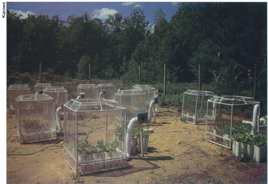
Using open-topped chambers like these at the University of Michigan Biological Station, scientists manipulate concentrations of carbon dioxide in the air.
